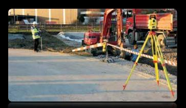
Leica iCON robot 50 is a versatile instrument that has your entire site covered. Data capture, control measurements, stake-out, machine control and as-built site verification can be completed quickly and easily.
